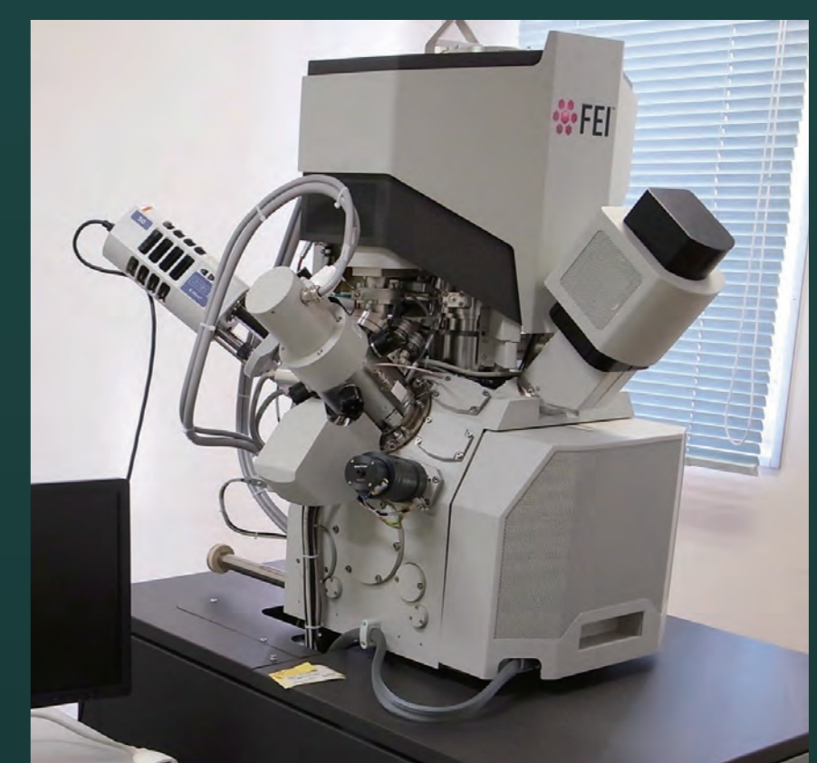
Analytical system: ATEM and FIB.
