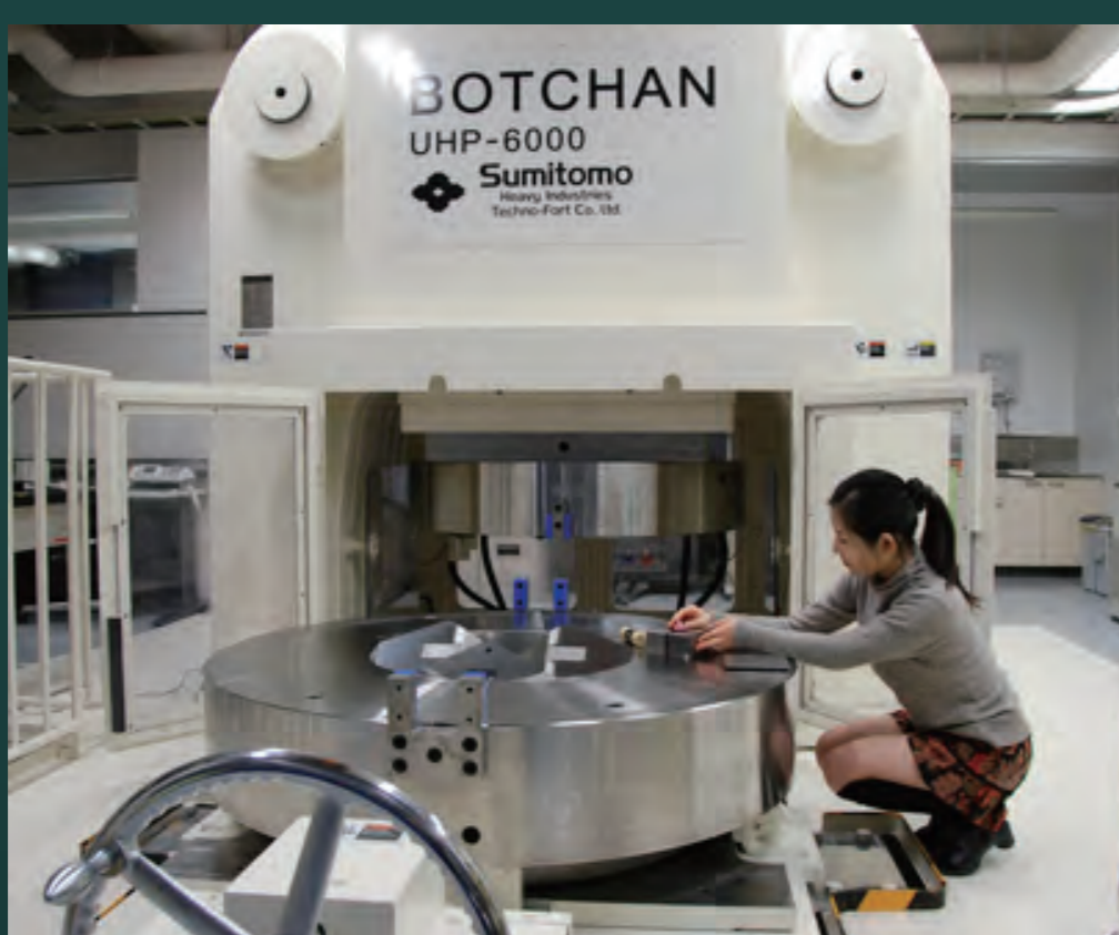
Multi-anvil apparatus (BOTCHAN, the world-largest press, 6000 tons).
